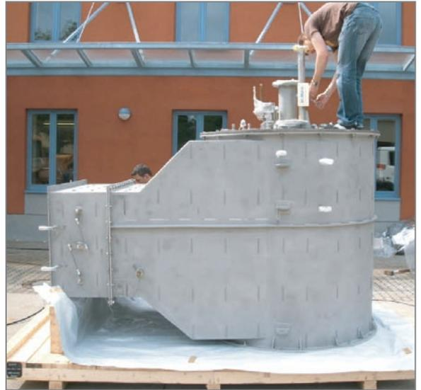
Sulphur burner with 2 heated sulphur lances, 3 gas lances and additional damper for combustion air for heating up with gas
